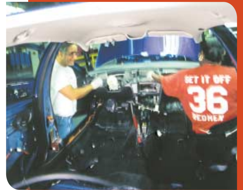
MOVING AHEAD: Above, Tom DiCintio and Michelle Colyar hook up the vent hose, route the heater control and set the dome light switch in place.
